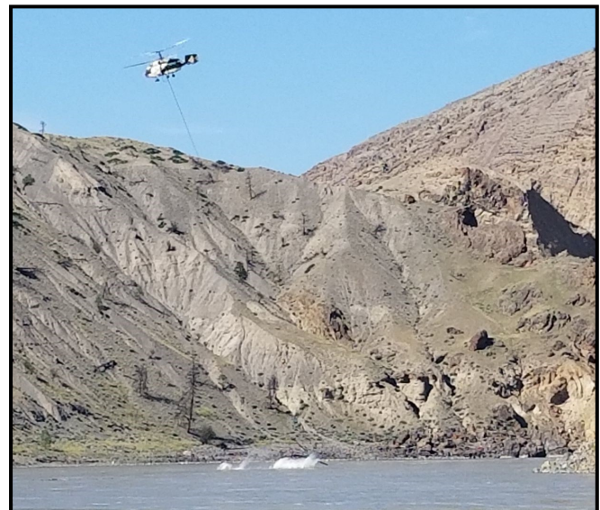
A heavy-lift helicopter removing unsafe woody debris with a logging grappling hook.
