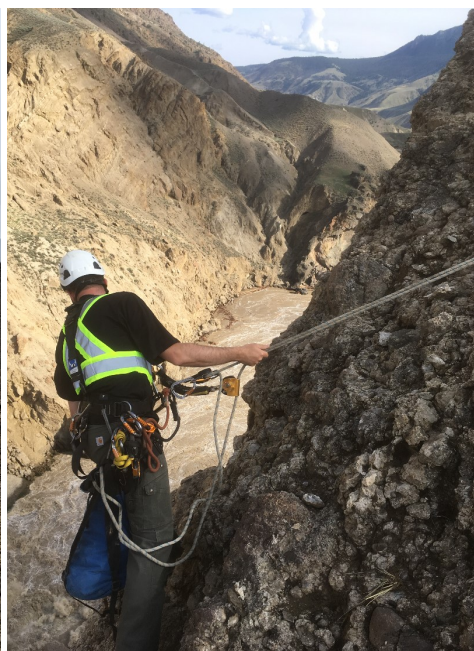
Engineering Geologist, Sam, uses a system of ropes and harnesses to safely assess the slide site.
